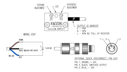
NOTE: Please use a fine tipped screwdriver and light touch when adjusting set point and hysteresis. Forcing the adjustment screw past its limits (270° max rotation) will damage the switch and void its warranty.
