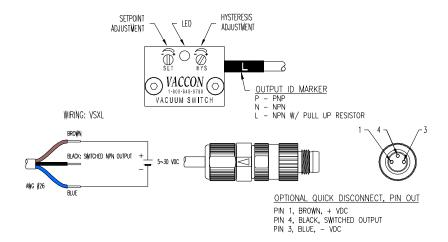
NOTE: Please use a fine tipped screwdriver and light touch when adjusting set point and hysteresis. Forcing the adjustment screw past its limits (270° max rotation) will damage the switch and void its warranty.
