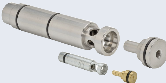
Top: Custom made C350H-303 stainless steel venturi cartridge 5.375" L x 1" dia. Bottom: Standard Mid Series C150H aluminum/brass cartridge is 2.2" L x 0.40" dia. Both cartridges generate up to 28"Hg.
